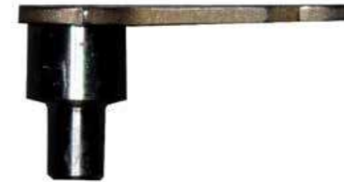
Fig. 9. Guide tube of 9 mm in length.
